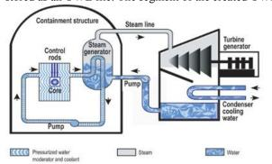
Figure 1. (a) Structure diagram of a nuclear power plant
