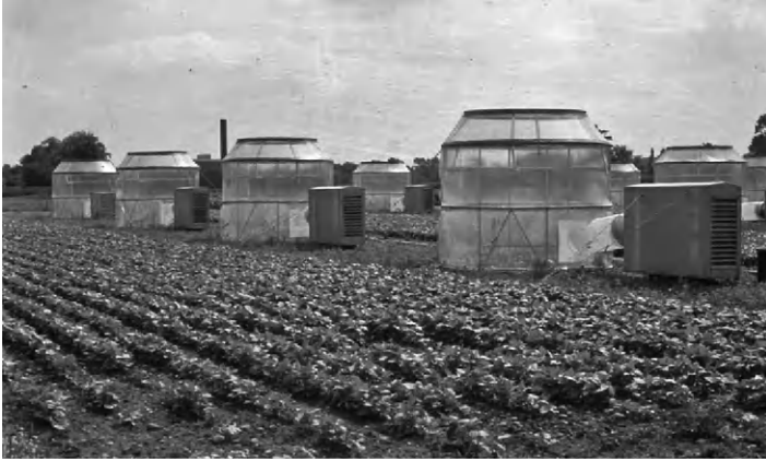
Figure 11.5 Open-top chambers in a field of beans at Sutton Bonington. The boxes adjacent to the chambers contained fans for ventilating the chambers, and some also contained charcoal filters for absorbing gaseous air pollutants. The “frustum” design at the open top reduced the rate of incursion of unfiltered air (see text).
