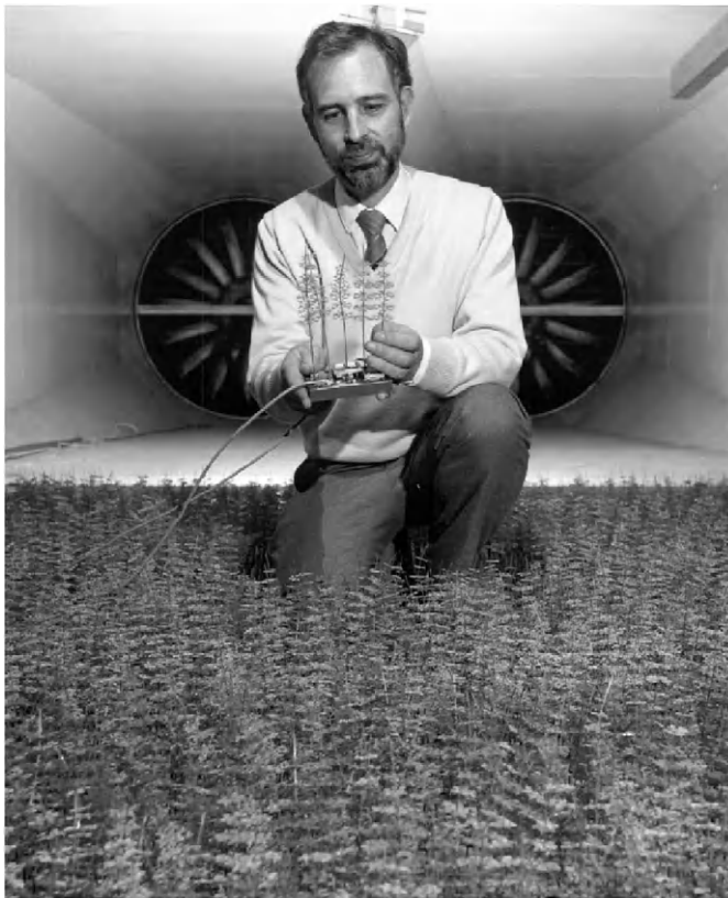
Figure 9.10 A wind-tunnel experiment using an array of model trees with realistically scaled properties. The researcher is holding an element of the array, showing how the trees are attached to strain gauges to measure wind forces (from Wood, 1995).
