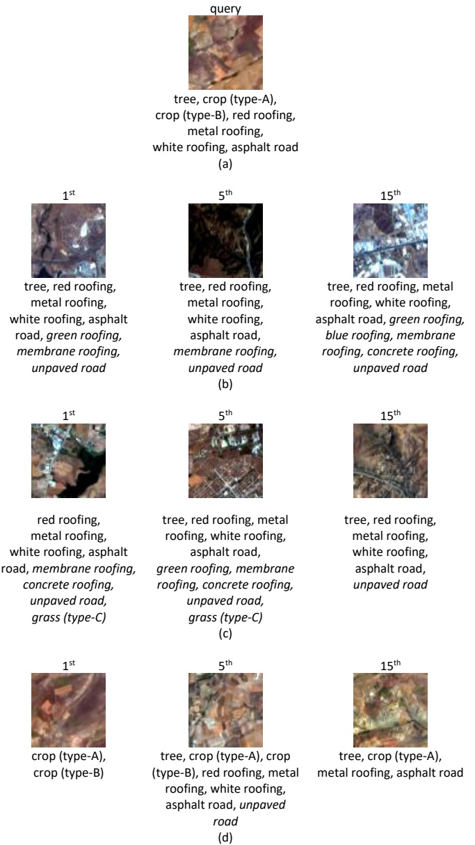
Fig. 11. Retrieval results from the Ankara archive: (a) query image, (b) images retrieved by the mSIFT-SVM, (c) images retrieved by the hybrid-SVM and (d) images retrieved by the proposed hybrid-SRR (corresponding multi-labels are reported below each image). Retrieved image labels that are not associated with the query image are given in italics.
