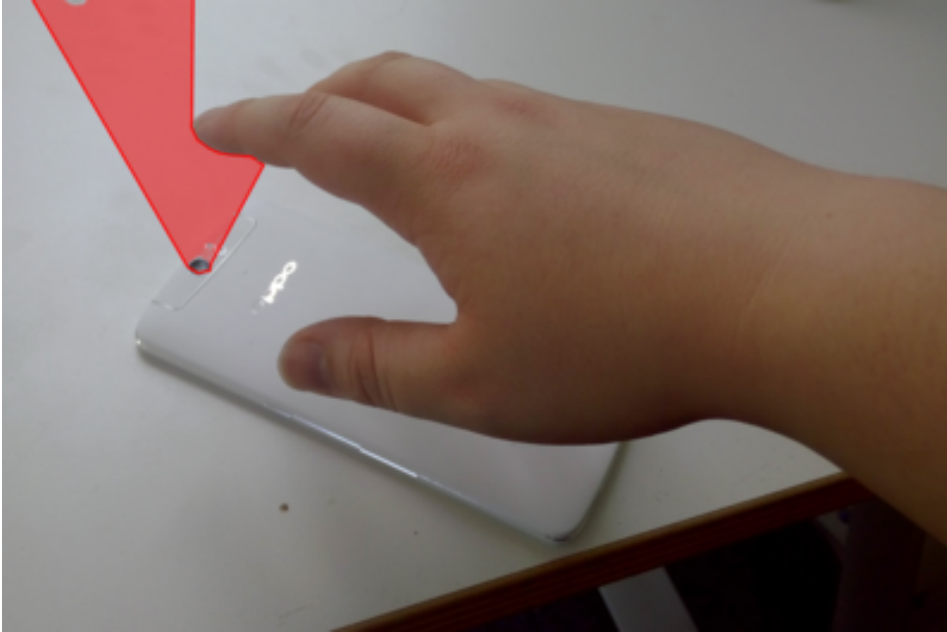
Figure 3.4: While a user picks up a device the right index finger moves through the rear-facing camera view-port (red). An attacker can use this moment to create an image of the user's fingerprints.
