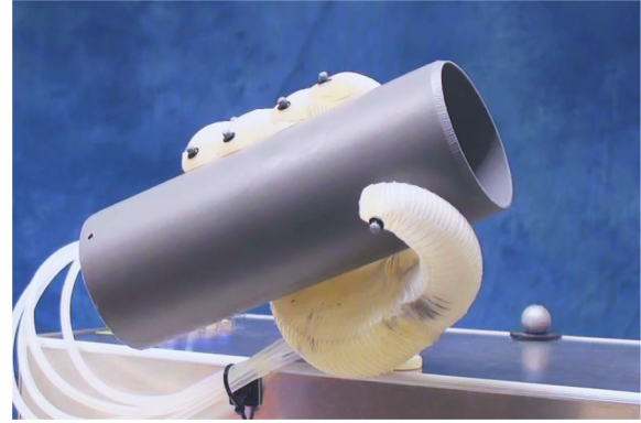
Fig. 16. Screen shot from video Extension 4, showing the marker placement on the fingertips for Motion Capture.
