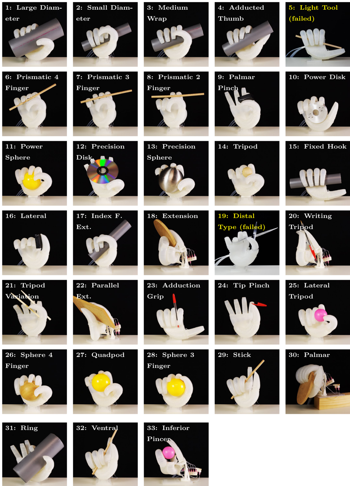
Fig. 12. Enacted grasps of the Feix taxonomy, using empirically determined actuation patterns: Grasps are numbered according to the Feix taxonomy (Feix et al., 2009); the hand failed to replicate grasps 5 (Light Tool) and 19 (Distal Type, Scissors).
