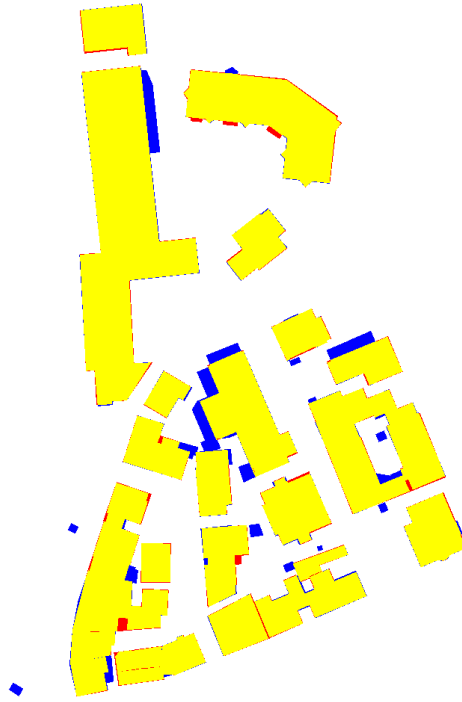
Figure 8.8. Evaluation result of the pixel-based building detection result (yellow: true positive pixels, blue: false negative pixels, and red: false positive pixels).
