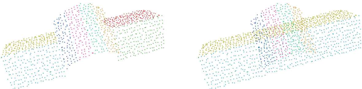
Figure 4.6. Segmentation of planar regions as a result of surface growing (left) and sub-surface growing (right).
