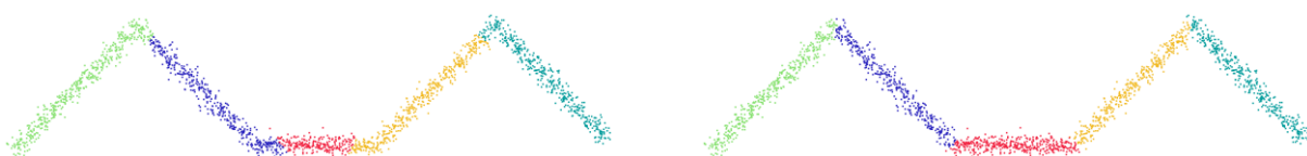
Figure 4.3. Segmentation results without (left) and with (right) reassignment of segment points; based on (Vosselman and Klein, 2010).
