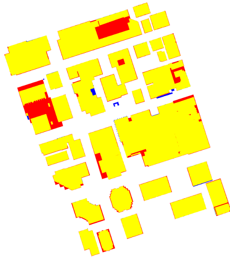
Figure 8.50. Evaluation result of the pixel-based building detection result (yellow: true positive pixels, blue: false negative pixels, and red: false positive pixels).
