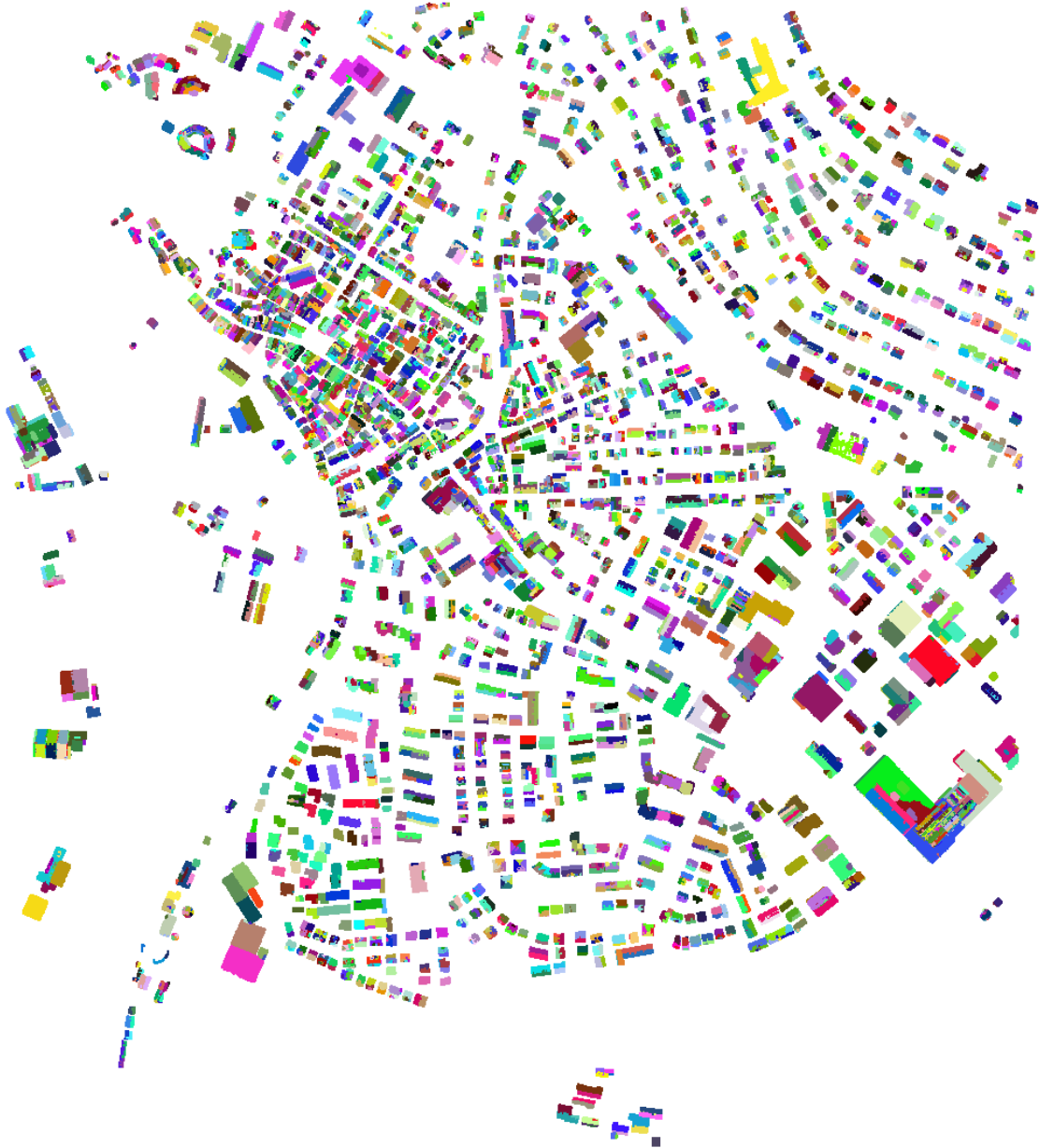
Figure 4.2. Segmentation result of surface growing performed on the Vaihingen data set.
