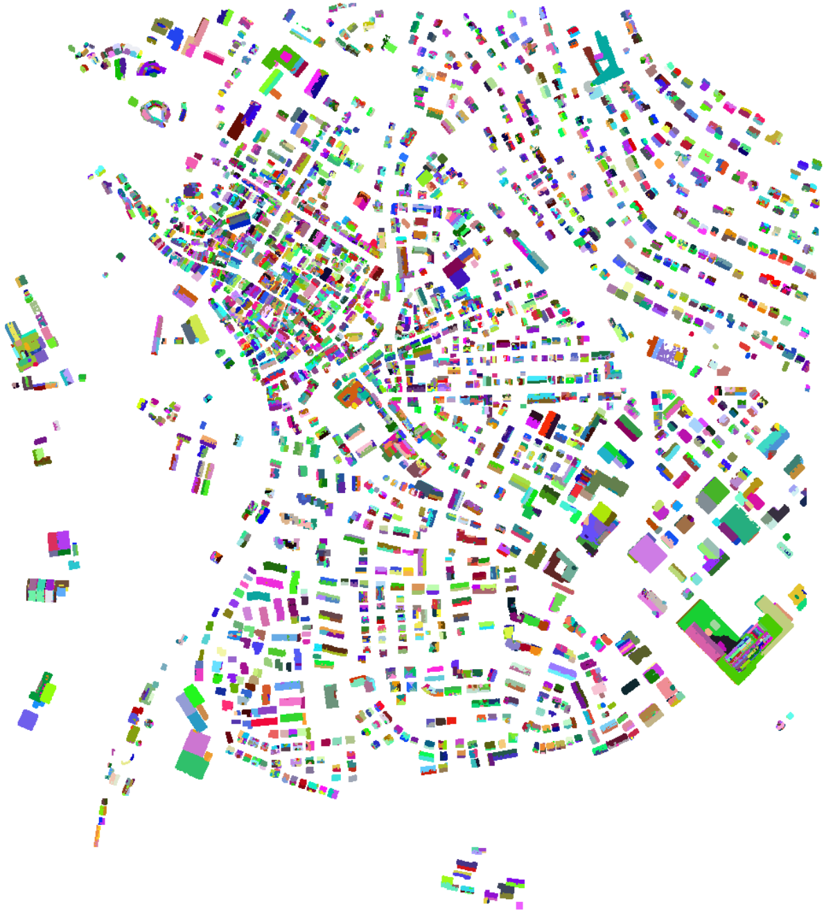
Figure 4.4. Segmentation result of sub-surface growing performed on the Vaihingen data set.
