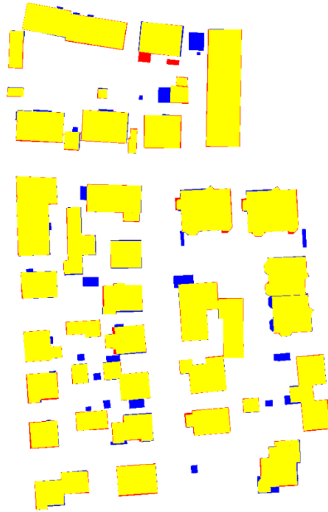
Figure 8.30. Evaluation result of the pixel-based building detection result (yellow: true positive pixels, blue: false negative pixels, and red: false positive pixels).
