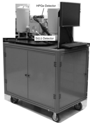
Figure 2: First Compact Compton Imager (CCI-1). The complete system including data acquisition mounted in the cart.
