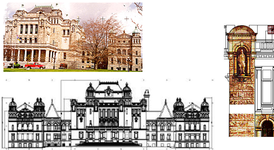
Figure 6: Full Architectural CAD Modeling by Terrestrial Photogrammetry
