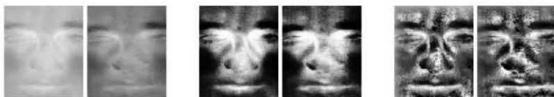
Figure 3: Comparison of e intensity normalization methods: original images are on the left; results of global histogram equalization are in the center, and results of local histogram equalization are on the right.
