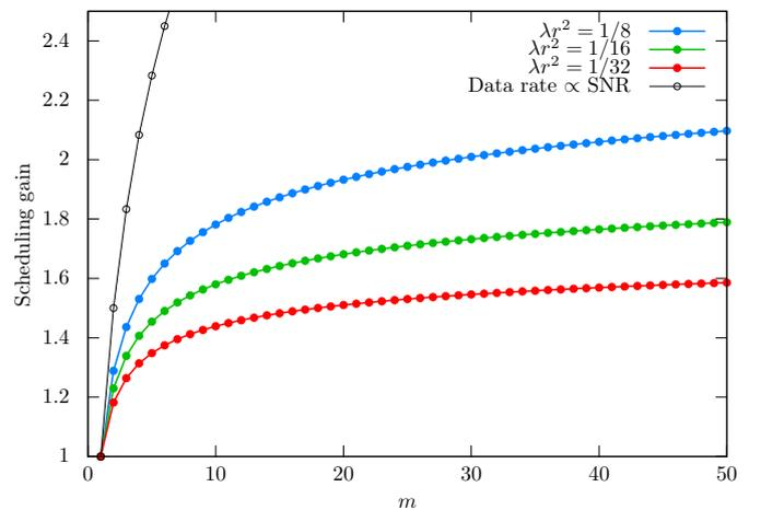
Fig. 3: Scheduling gain in multiuser extended Poisson bipolar networks for  $\alpha = 4$ .
