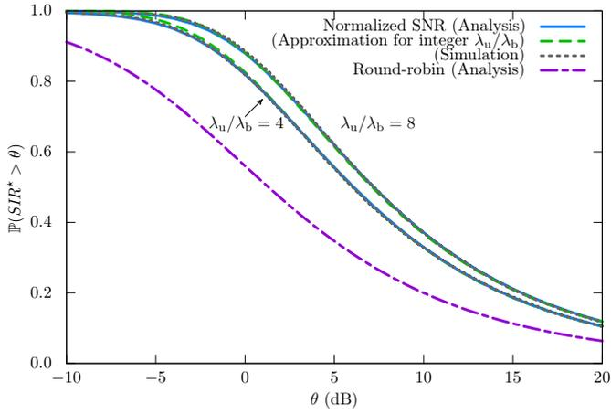
Fig. 5: SIR ccdf in Poisson cellular networks for  $\alpha = 4$ .
