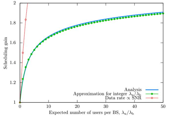
Fig. 6: Scheduling gain in Poisson cellular networks for  $\alpha = 4$ .
