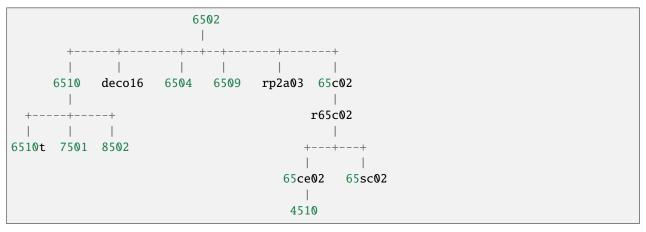
The 6510 adds an up to 8 bits I/O port, with the 6510t, 7501 and 8502 being software-identical variants with different pin count (hence I/O count), die process (NMOS, HNMOS, etc.) and clock support.
