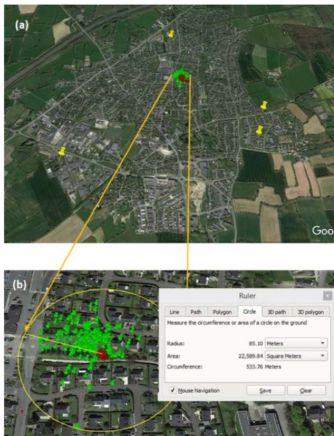
Figure 5-17: (a) Thorigné-Fouillard LoRaWAN network testbed (b) estimated positions for a stationary end-device
