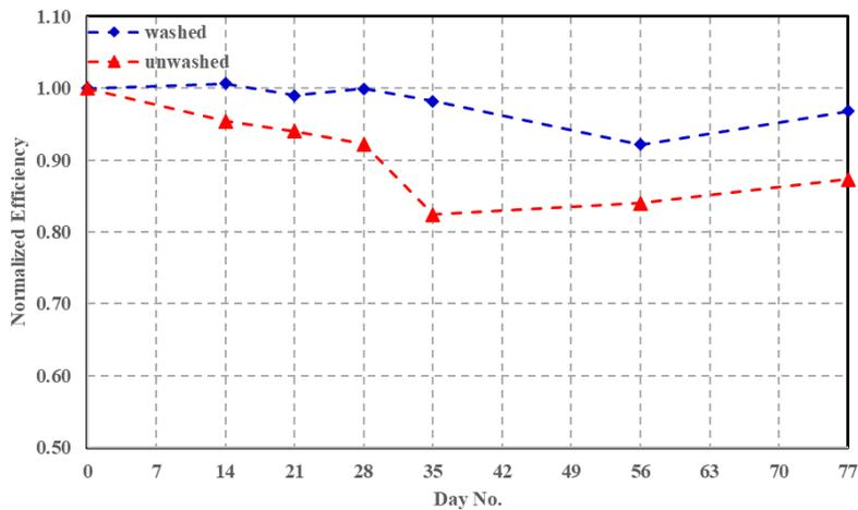
Fig.7: Normalized Efficiency Vs Time at Constant Irradiance of 850W/m<sup>2</sup>
