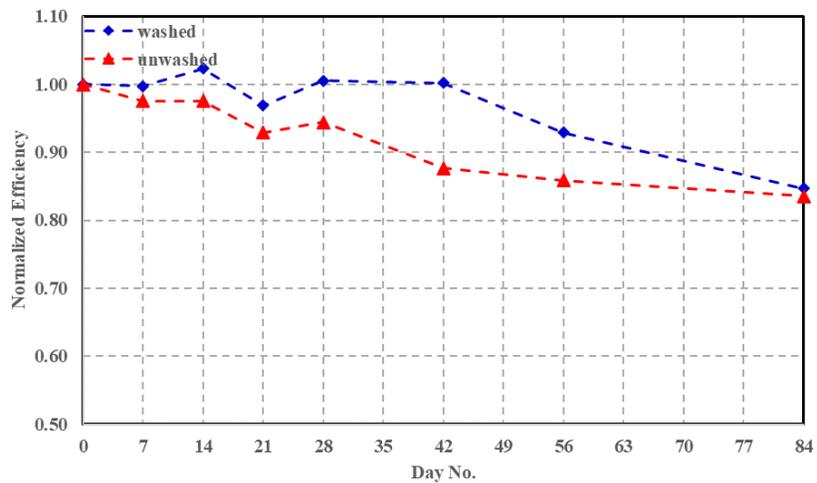
Fig.8: Normalized Efficiency Vs Time at Constant Irradiance of 900W/m<sup>2</sup>
