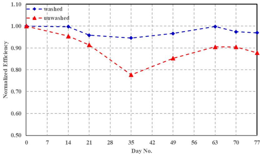
Fig.5: Normalized Efficiency Vs Time at Constant Irradiance of 750W/m<sup>2</sup>
