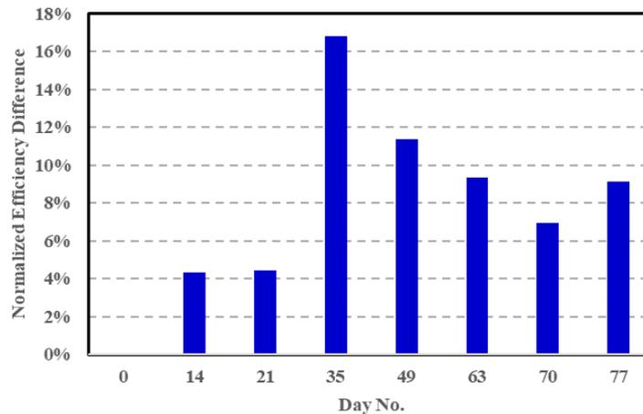
Fig.9: Normalized Efficiency Difference Vs Time at Constant Irradiance of 750W/m<sup>2</sup>
