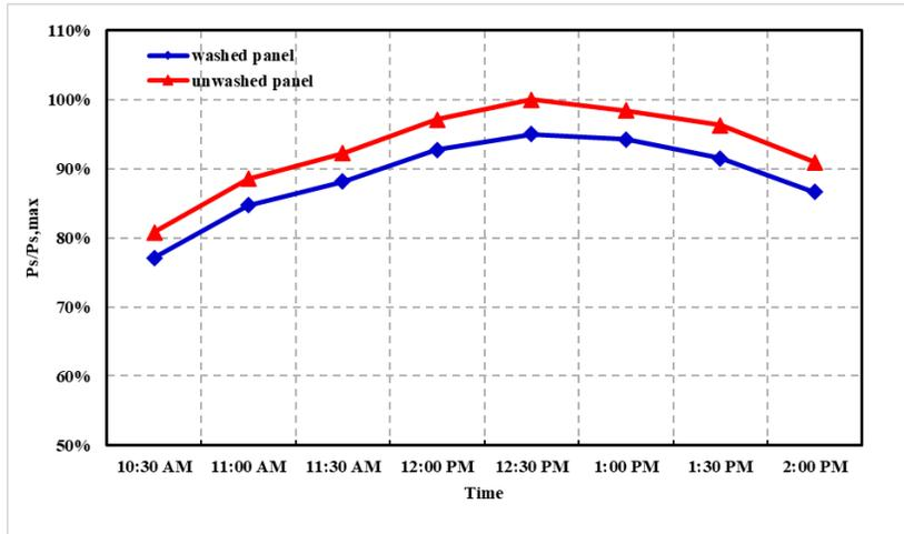
Fig.4: Panels Power Output Normalized by the Maximum Power Output
