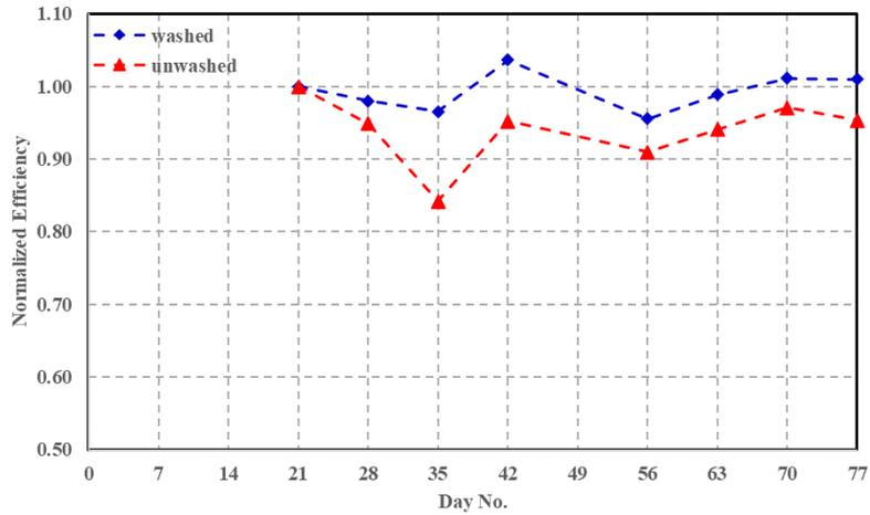
Fig.6: Normalized Efficiency Vs Time at Constant Irradiance of 800W/m<sup>2</sup>
