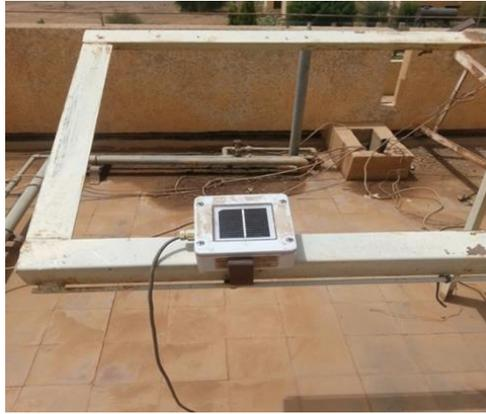
Fig.2: Pyranometer SOZ-03 Inclined at an Angle of 15.5° Facing South.
