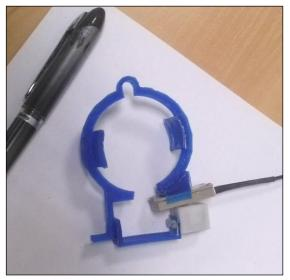
**Fig.7.** Horizontal strains sensor (its holder was designed and manufactured on a three-dimensional printer) based on Hall effects dedicated for a specified sample size
