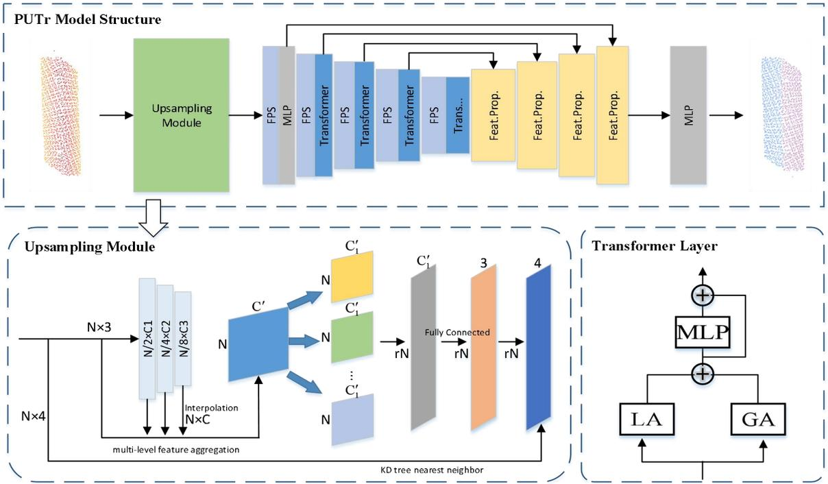
Figure 1. The Overall Architecture Of PUTr
