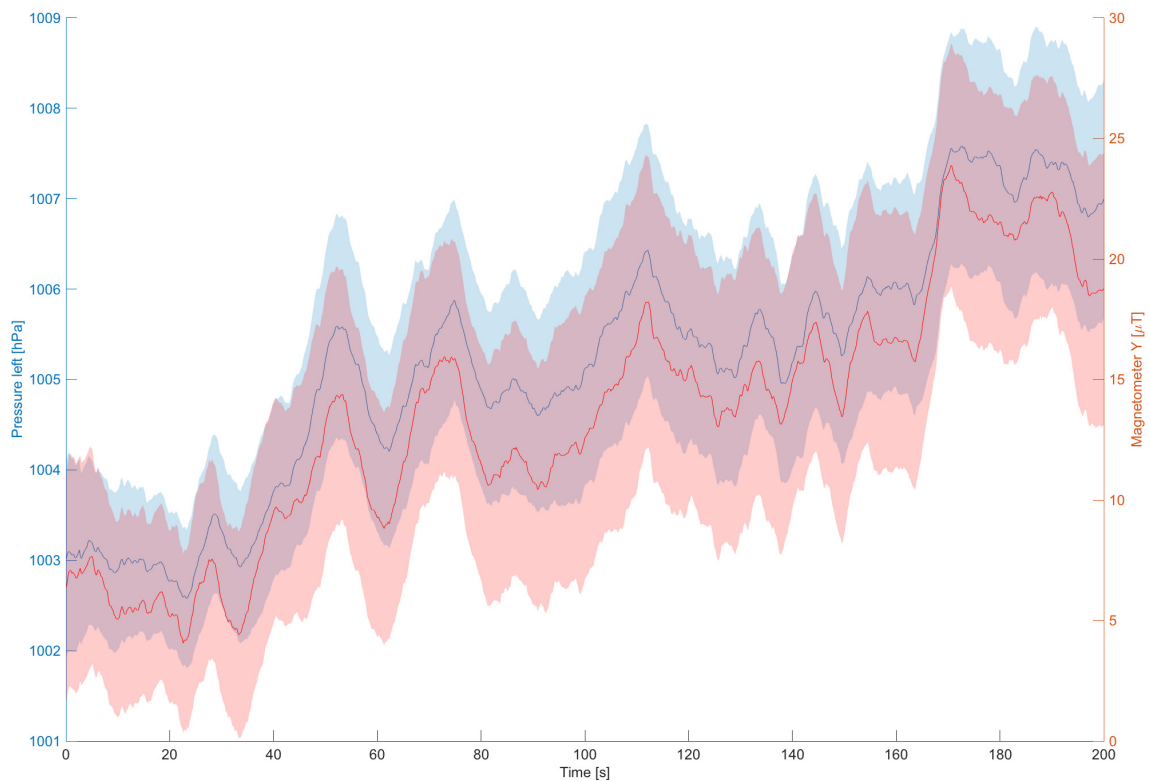
Figure 7. Left pressure and magnetometer in y-direction time series. The plot shows the first 200 seconds of 40 deployments ( n=40 ), with a moving mean with a time window of 5 s and the 95% confidence interval (shaded area).
