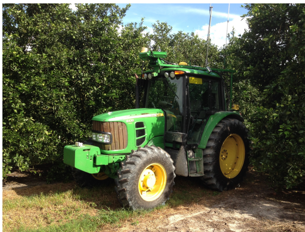
Figure 1. Tractor with stereo camera setup for motivating application.
