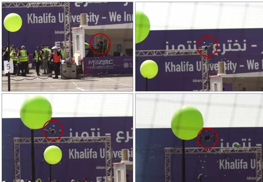
Figure 15. Image sequence of popping the first balloon in the Grand Challenge. Jelly (marked with the red circle) (1) takes off to 4.0 m. (2) After detecting the first balloon, the robot targets a position 2.0 m behind and 0.7 m above balloon's center. (3) It further accelerates to pass through the balloon with significant velocity. (4) It successfully pops the balloon. The entire shown process only takes 4.9 s.
