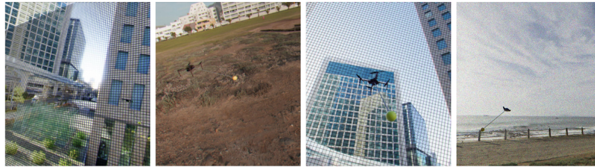
Figure 17. Synthetic training images for target detection of drone and yellow ball.
