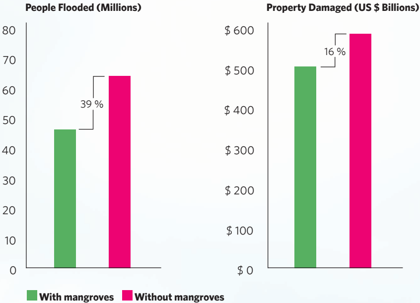
Figure 3: The bars show the global annual expected damages from flooding with current mangroves and without mangroves, including percent damages currently averted by mangroves.
