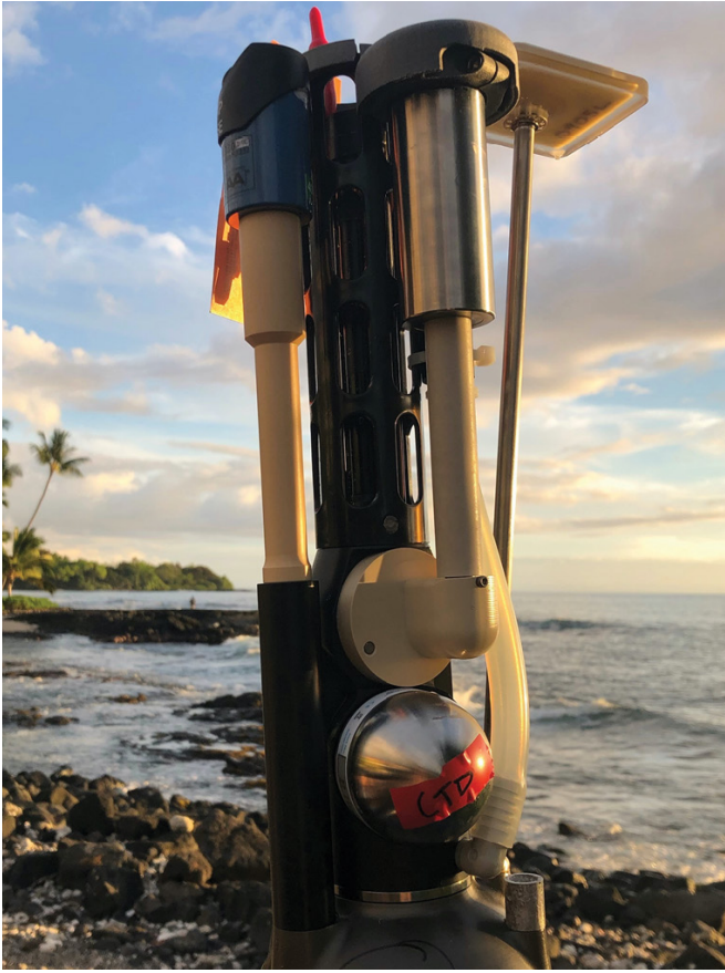
An Argo float equipped with newly developed oxygen sensors, pictured prior to deployment in the tropical Pacific Ocean, November 2020. Credit: NOAA.
