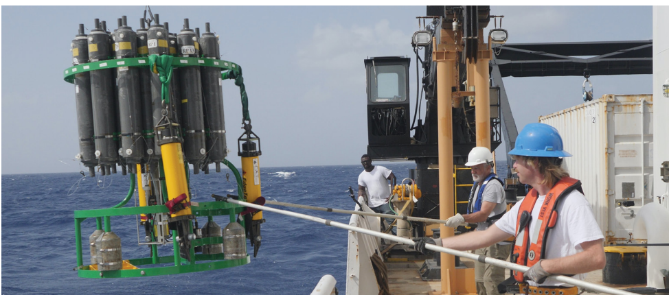
Deploying a Climate, Temperature, and Depth Rosette, which measures temperature and salinity of sea water at different depths, as part of the NOAA-led Atlantic Tradewind Ocean-atmosphere Mesoscale Interaction Campaign (ATOMIC). Credit: Richard Marchbanks, CIRES/NOAA.
