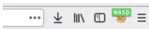
FIGURE 5.12: Firefox toolbar indicating archiving is activated. The context-menu of this icon allows to turn off the proxy-usage, thereby implementing a “pause-archiving” button.
