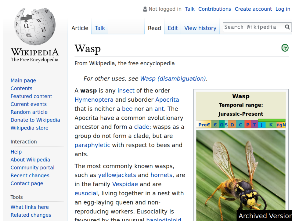
FIGURE 5.9: Screenshot of a web page reproduced from the archive. pywb is configured to insert a small black banner at the bottom right of the browser viewport to remind users that they are viewing an archived page.
