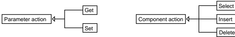
Figure A.10. All kinds of modifications must be put down to the five basic action types shown in the figure.
