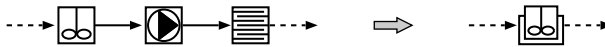
Figure 3.7. Replacement of a partial chain consisting of a mixer, a pump, and a heat transfer unit by a mixer device with built-in heat transfer. Again, the dashed lines stand for a variable number of edges. For the sake of simplicity edge labels have been omitted.
