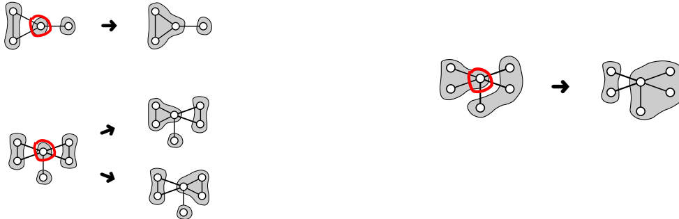
Figure 4. Illustration of Step 6+7 in MAJORCLUST: A definite majority decision (left top), and an indefinite decision (left bottom) when assigning a single node to a cluster. The right-hand side shows a situation where a node changes its cluster.
