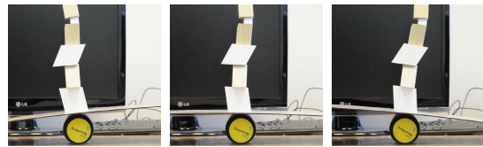
Figure 12: Testing a block stack generated under the constraint that it be stable at up to \pm 10^\circ tilts of the ground plane.
