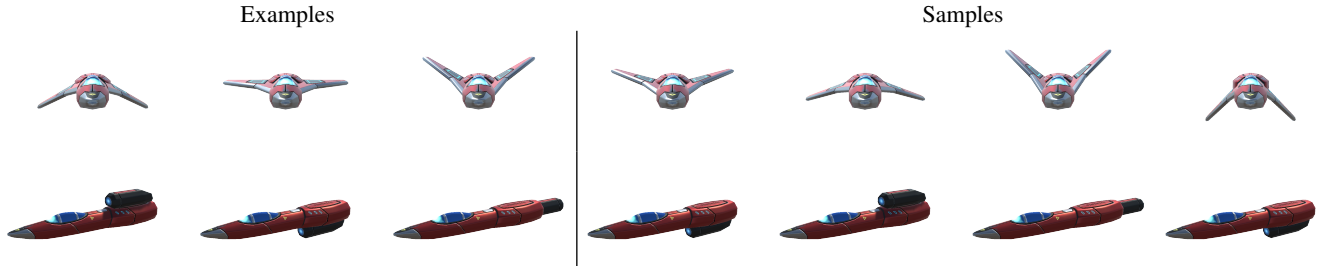
Figure 4: A toy example illustrating our learnable program’s ability to model continuous variability. (Top): Given three examples with wings in a range of configurations, the program learns to generate output samples which interpolate between and extrapolate from the example configurations. (Bottom): The three examples put the engine in completely different configurations, and the program learns to use a separate abstraction for each of these configurations.
