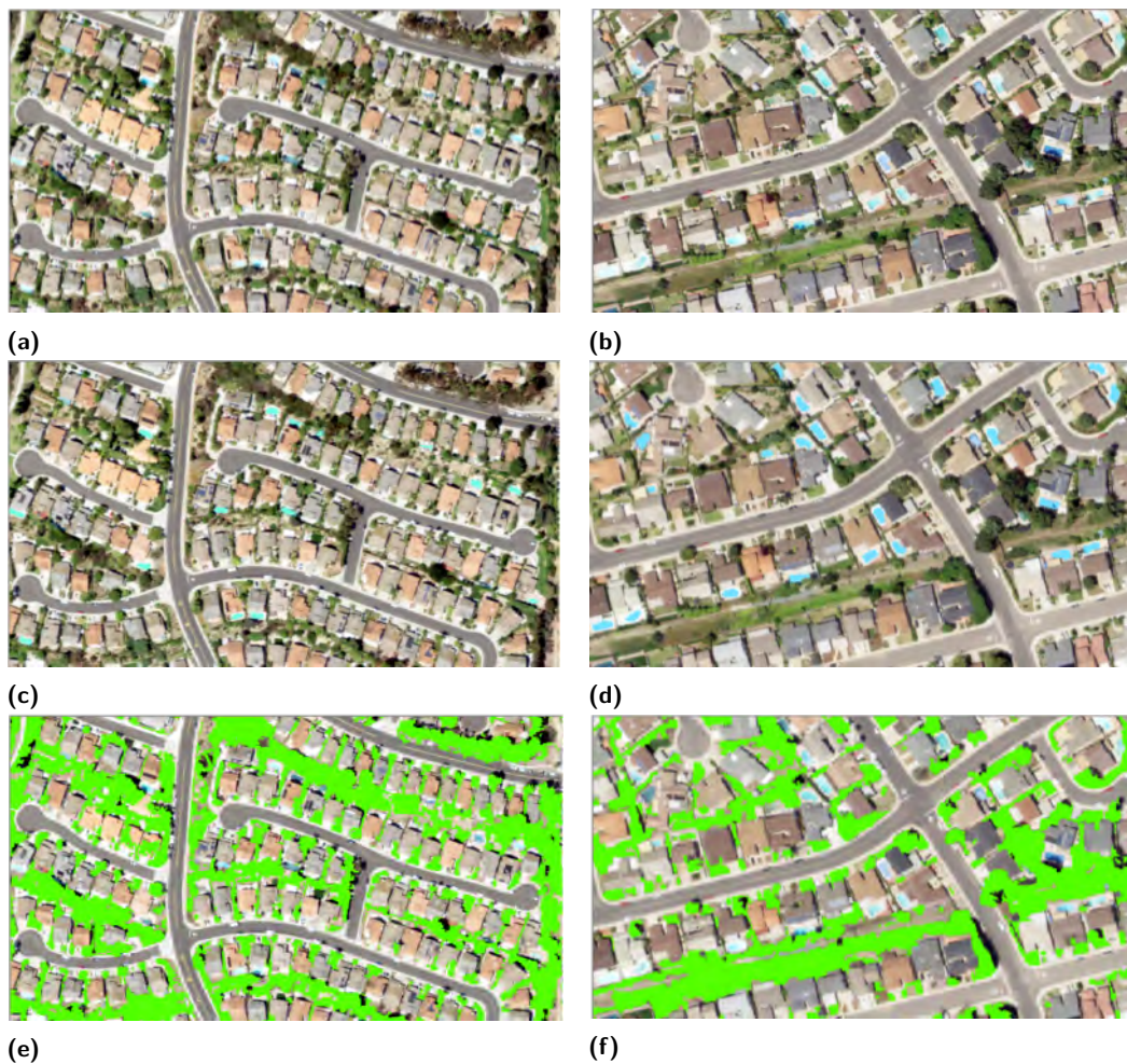
■ Figure 1 The NAIP image with the detection of vegetation cover and swimming pools in high SES and medium SES in San Diego County.
