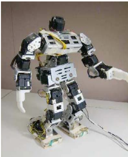
Figure 5. Cycloid II robot with pressure sensors added to foot pads and tether to PC.
