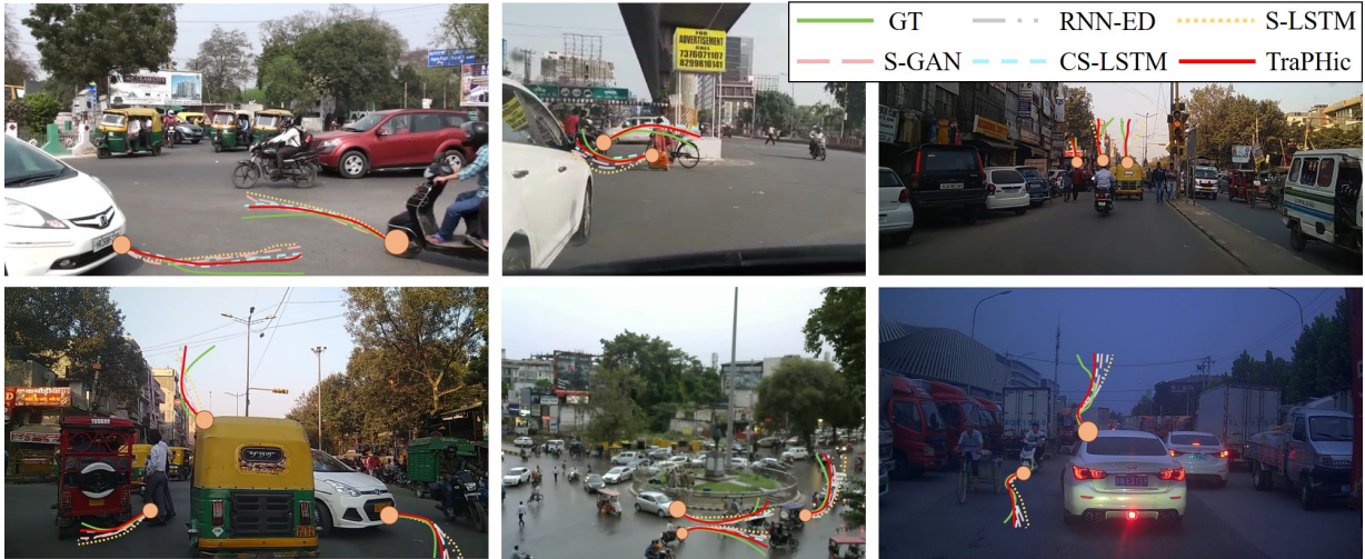
Figure 2.9: Trajectory Prediction Results: We highlight the performance of various trajectory prediction methods on our TRAF dataset with different types of road-agents. We showcase six scenarios with different density, heterogeneity, camera position (fixed or moving), time of the day, and weather conditions. We highlight the predicted trajectories (over 5 seconds) of some of the road-agents in each scenario to avoid clutter. The ground truth (GT) trajectory is drawn as a solid green line, and our (TraPHic) prediction results are shown using a solid red line. The prediction results of other methods (RNN-ED, S-LSTM, S-GAN, CS-LSTM) are drawn with different dashed lines. TraPHic predictions are closest to GT in all the scenarios. We observe up to 30% improvement in accuracy over prior methods over this dense, heterogeneous traffic.
