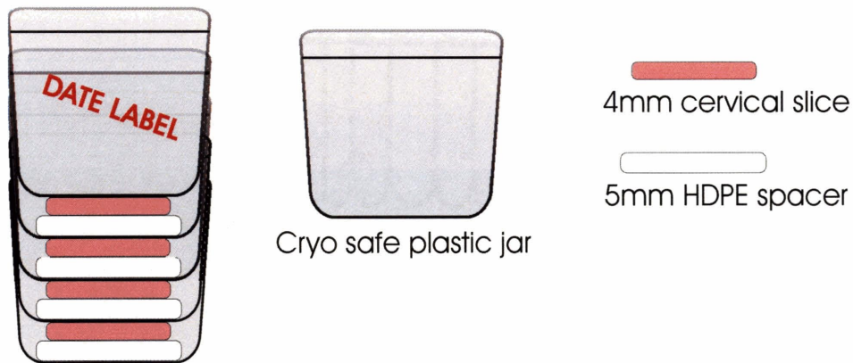
Figure 2-2: Plastic device used to store cervical slices.
