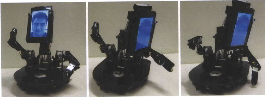
Figure 2-17: A picture that shows multiple views of the MeBot V4 (The blue tone is an artifact of the still image, the colors are in fact correct).
