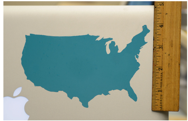
Figure 9: Fine details: With a vinyl cutter, the resolution of features is not limited by the width of the bit. Here, we show a 6"-wide sticker with fine details.
