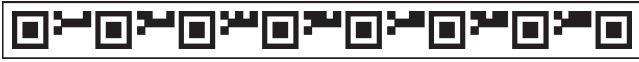
Figure 3: Markers: A sequence of markers, with values 1000 to 1006, such as would be printed on a strip of tape. In our current implementation, markers are printed at a size of roughly 0.8'' \times 0.4'' . This is small relative to the area of the material the camera can see at once (roughly 8'' \times 6'' ).
