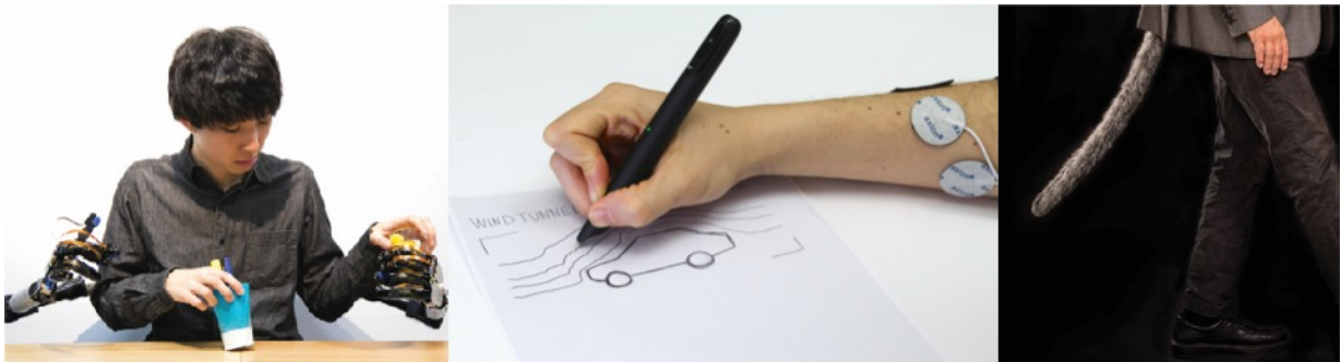
Figure 1. Exemplars of Human-Computer Integration: extending the body with additional robotic arms; [70] embedding computation into the body using electric muscle stimulation to manipulate handwriting [48]; and, a tail extension controlled by body movements [86].
