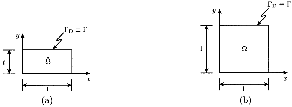
Figure 3-3: Example 3: (a) Parameter-dependent rectangular domain with internal heat source; and (b) a reference domain.
