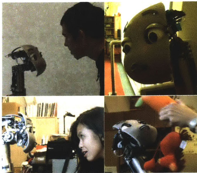
Figure 1-1: Mertz is an expressive head robot designed to explore incremental individual recognition through natural interaction. The robot's task is to learn to recognize a set of familiar individuals in an incremental and unsupervised fashion.
