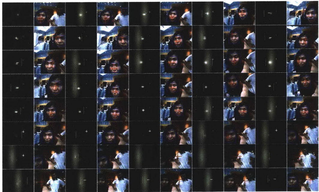
Figure 4-17: A snapshot of the attention output while the robot maintained a short-term memory for a person while interacting with another person.
