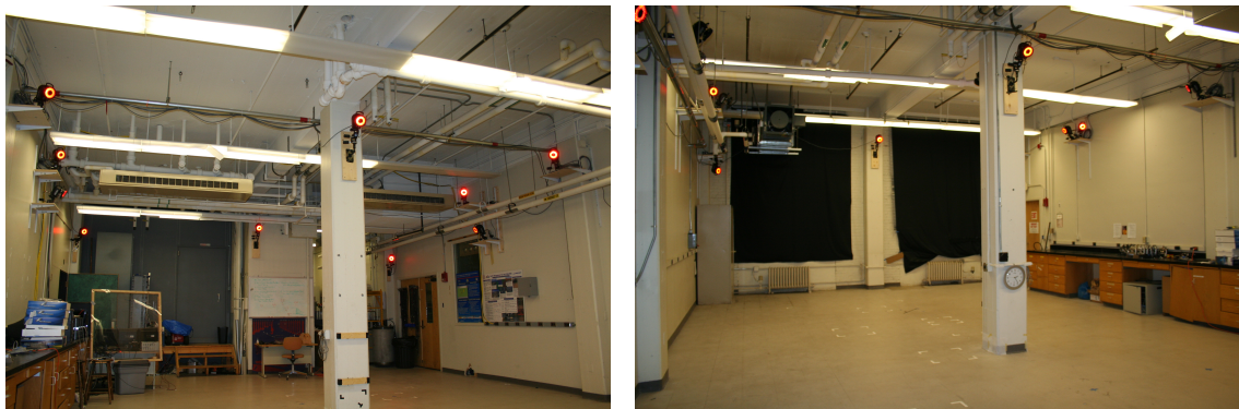
Figure 1-3: MIT's Real-time indoor Autonomous Vehicle test ENvironment (RAVEN) showing the Vicom motion capture camera system.
