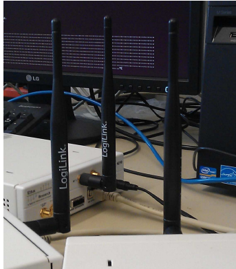
Figure 4.3: IA testbed setup: Demonstration of the antennas within one transmitting node.
