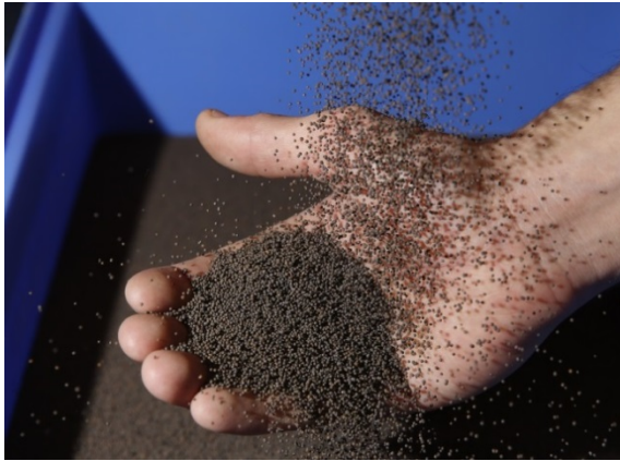
Figure 3: Solid bauxite particles used as HTM
