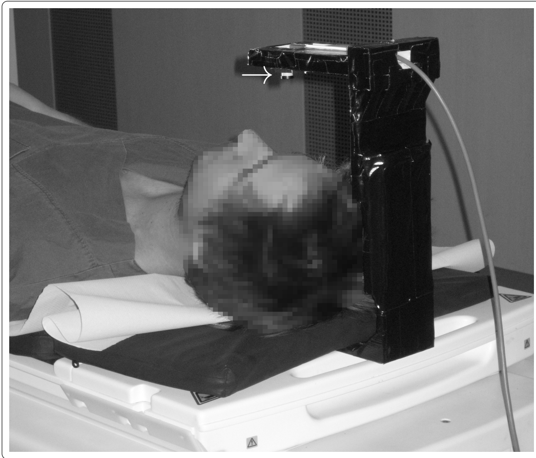
Figure 3.1: Experimental setup during stage ①: The patient is lying feet-first on the patient table and the camera (arrow) is pointed towards the forehead. The camera is mounted on a MR-compatible custom-built stand . During stages ② and ③ the setup remains identical but the patient table is located at the isocenter of the scanner.
