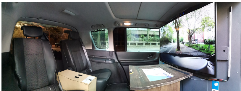
Figure 3.2: View into the passenger cabin – the cabin TV projects the camera view from the windshield into the passenger cabin.
