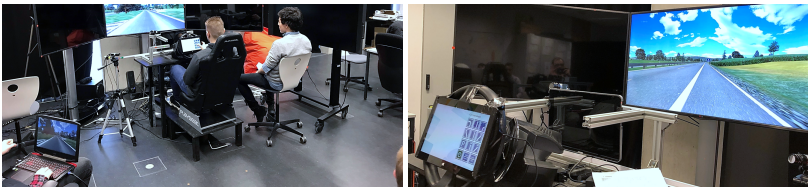
Figure 7.7: Experimental Setup – The wizard simulated the system while the participant sits in the driving simulator's primary seat and the visible researcher next to her or him.
