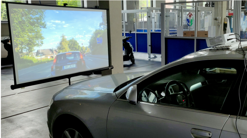
Figure 9.5: Video study setup – A stationary car and the projection of the real-world driving video augmented with CGI-visualizations of the HUD concepts on canvas.
