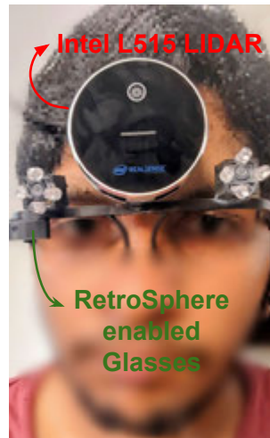
Fig. 11. Experimental setup of RetroSphere-enabled glasses-like prototype attached with an Intel L515 LIDAR sensor for ground truth 3D measurements.
