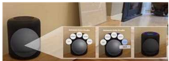
Figure 13: XR-OBJECTS detects devices, such as speakers, and provides custom UI elements for IoT control.
