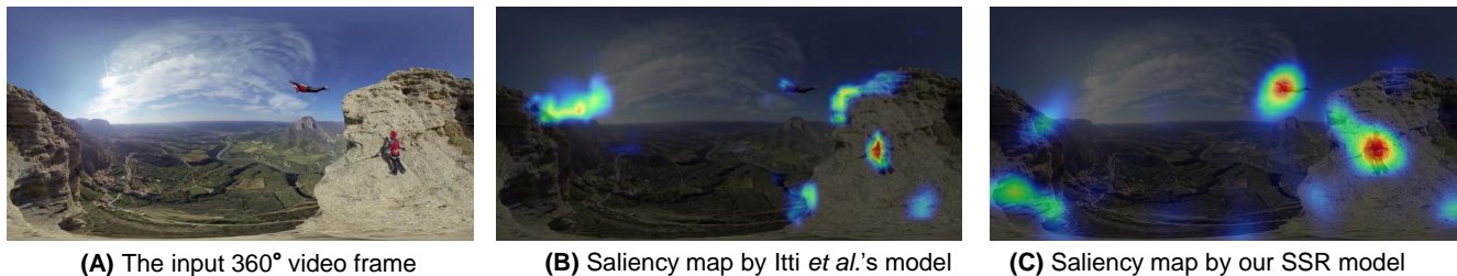
Figure 1: This paper presents an efficient GPU-driven pipeline of computing saliency maps of 360° videos using spherical harmonics (SH). (A) shows an input frame from a 360° video. (B) shows the saliency maps computed by the Itti model in 104.46 ms on the CPU. (C) show the saliency maps computed by our spherical spectral residual (SSR) model in 21.34 ms on the CPU and 10.81 ms on the GPU. In contrast to the Itti model, our model is formulated in the \mathbb{SO}(2) space and handles challenging cases such as horizontal clipping, spherical rotations, and equator biases in 360° videos.
