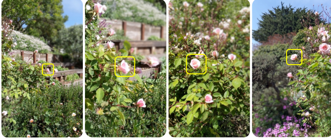
Figure 13. Wide-aperture effect focused on a world-anchored point on a flower from different perspectives. Unlike traditional photography software, which only anchors the focal plane to a screen point, DepthLab allows users to anchor the focal point to a physical object and keep the object in focus from even when the viewpoint changes. Please zoom in to compare the focus and out-of-focus regions.
