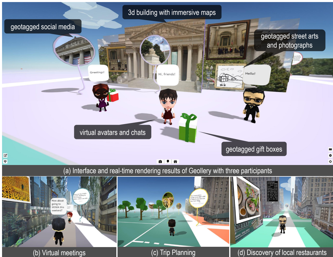
Figure 1.3: Interface, rendering results, and use cases of Geollery (a) shows the interface and real-time rendering results of Geollery with three participants. Geollery progressively fuses 3D buildings, virtual avatars, and geotagged social media into a mirrored world. (b), (c), and (d) show three potential applications: virtual meeting, trip planning, and discovery of local business and events.
