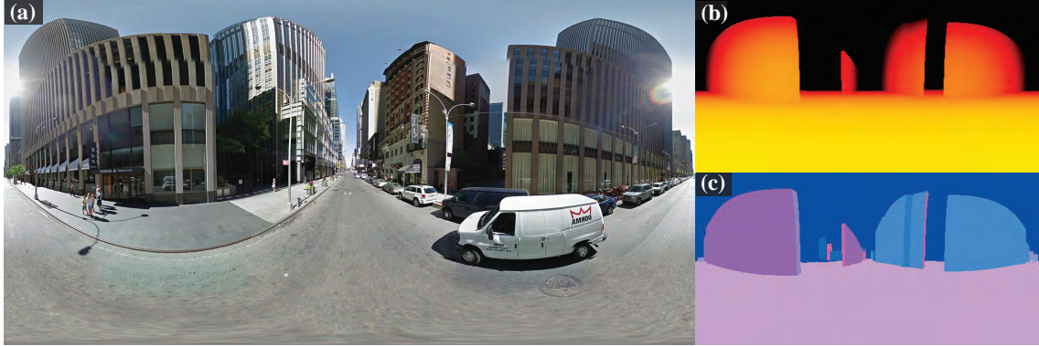
Figure 2.4: The illustration of (a) stitched panoramic image tiles, (b) depth map and (c) normal map from Google Street View. The depth map is visualized in a yellow-red-black color scheme, where black indicates 255 meters or more, red indicates 128 meters and yellow indicates 0 meters. The normal map contains a 3D normal vector for each pixel. We visualize the normal data by converting the normal vector to HSV color space with blue-purple hues.
