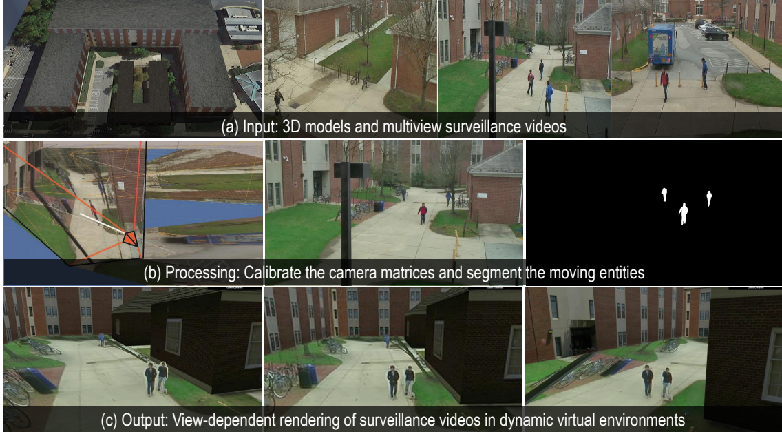
Figure 1.6: Video Fields system fuses multiple videos, camera-world matrices from a calibration interface, static 3D models, as well as satellite imagery into a novel dynamic virtual environment. Video Fields integrates automatic segmentation of moving entities during the rendering pass and achieves view-dependent rendering in two ways: early pruning and deferred pruning. Video Fields takes advantage of the WebGL and WebVR technology to achieve cross-platform compatibility across smart phones, tablets, desktops, high-resolution tiled curved displays, as well as virtual reality head-mounted displays. See the supplementary video at http://videofields.com
