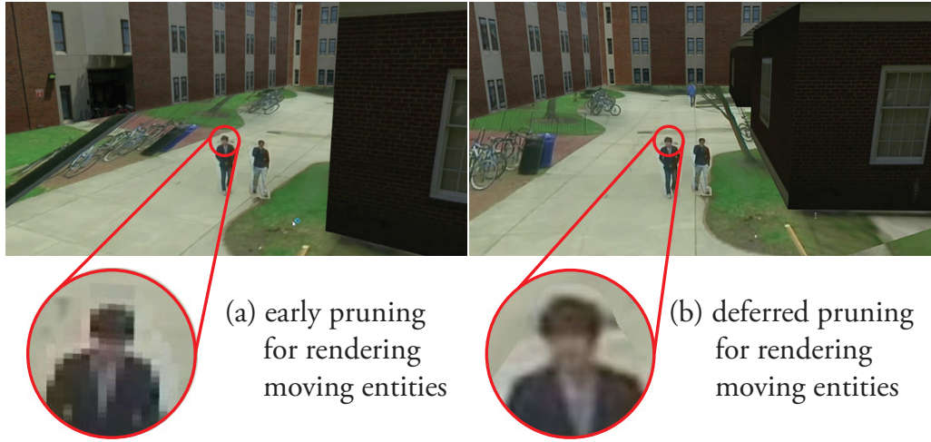
Figure 4.7: This figure shows the segmentation of moving entities, view-dependent rendering, as well as zoom-in comparison between the early pruning algorithm and the deferred pruning algorithm.
