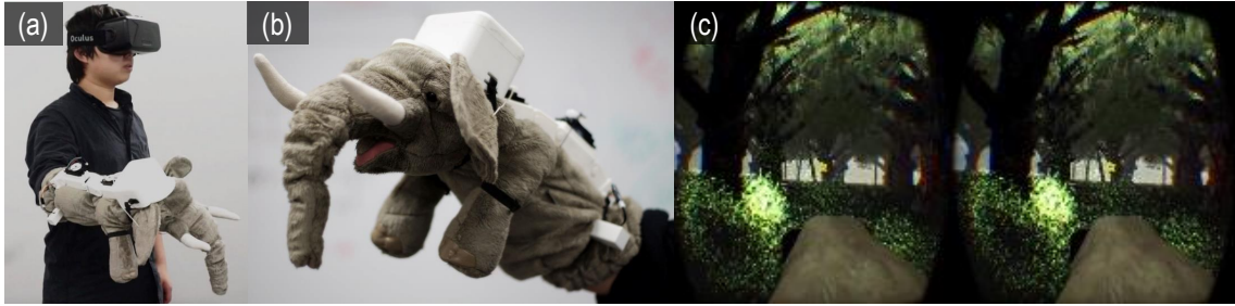
Figure 5.1: Overview of VRSurus . (a) a puppeteer wearing an elephant puppet with VRSurus playing a VR game, (b) shows a closer view of the elephant puppet wearing a custom 3D-printed cap that encapsulates the Arduino microcontroller, an inertial measurement unit and other electronic modules, and (c) shows the educational VR game empowered with gesture recognition and tactile feedback.
