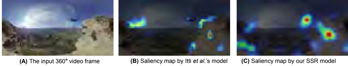
Figure 3.1: This chapter presents an efficient GPU-driven pipeline of computing saliency maps of 360° videos using spherical harmonics (SH). (A) shows an input frame from a 360° video. (B) shows the saliency maps computed by the classic Itti et al. 's model in 104.46 ms on the CPU. (C) show the saliency maps computed by our spherical spectral residual (SSR) model in 21.34 ms on the CPU and 10.81 ms on the GPU. In contrast to the classic models for images in rectilinear projections, our model is formulated in the \mathbb{SO}(2) space. Therefore, it remains consistent in challenging cases such as horizontal clipping, spherical rotations, and equator biases in 360° videos.
