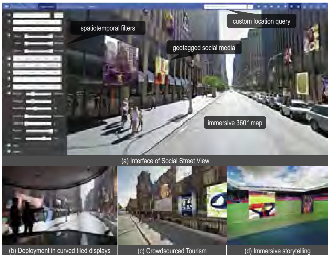
Figure 1.1: Interface, deployment, and use cases of Social Street View . (a) shows the graphic user interface of Social Street View . Given a custom location query with spatiotemporal filters, our system automatically fetches geotagged social media from Twitter and Instagram and immersive maps from Google Street View . The social media images are aligned with building geometry and laid out aesthetically with the immersive map. (b) shows the deployment in an immersive curved screen environment with 15 projectors. Users can interactively explore hundreds of social media messages near a New York City street with a game controller at a resolution of 6K \times 3K pixels. (c) shows a use case for crowdsourced tourism, where users can look through the museum in Paris for geotagged artworks inside as well as the dishes in nearby restaurants. (d) shows an example for immersive storytelling, where geotagged photographs of a football game are embedded into the 360° stadium where the event occurred. Please refer to the supplementary materials at http://socialstreetview.com for more examples.
