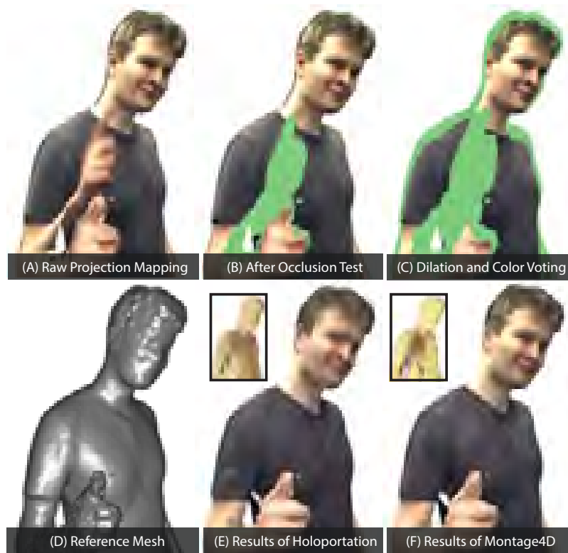
Figure 6.3: This figure shows how texture weight fields improve the rendering quality compared to previous work (the baseline approach). The Holoportation approach removes several ghosting artifacts by taking advantage of dilated depth maps and majority voting algorithm (top row), however, the rendering still suffers from fuzziness and visible seams (bottom row). (A) shows the raw projection mapping result from an input video texture, (B) shows the culling result after the occlusion test, (C) shows the culling result after using dilated depth maps and majority voting algorithm, (D) shows the input mesh, (E) and (F) respectively shows the rendering results from the baseline approach and our algorithm, together with the corresponding texture weight fields for comparison.
