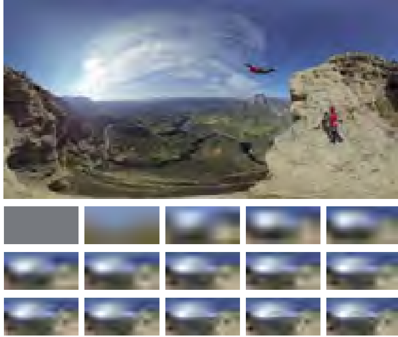
Figure 3.3: The reconstructed images with the first 15 bands of spherical harmonics coefficients extracted from the video frame.
