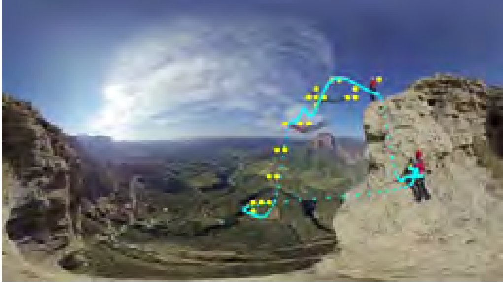
Figure 3.7: This figure shows the interpolation amongst the global maximums of the saliency maps in the spherical space. The yellow dots show the discrete optimal location using the energy function, and the blue dots show the interpolation using the spherical spline curve with C^2 continuity.
