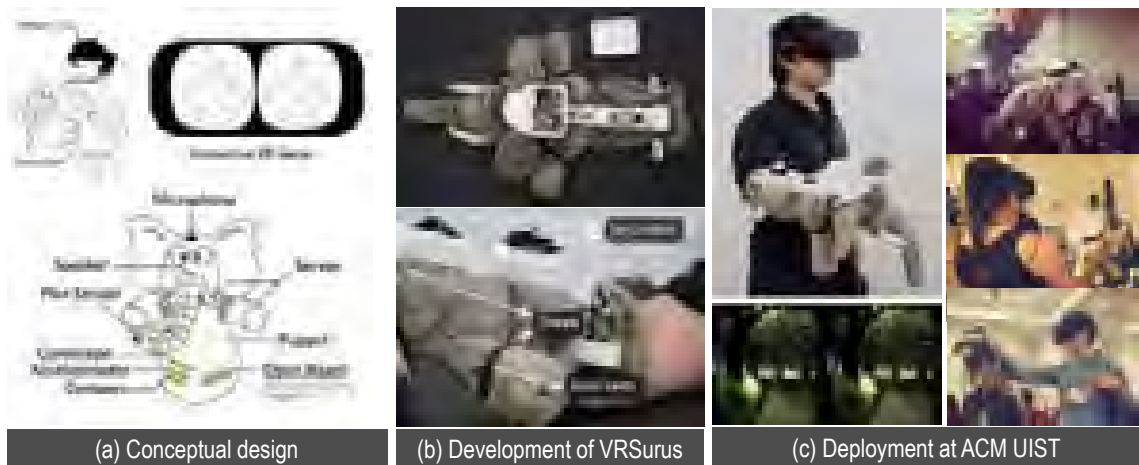
Figure 1.7: (a) shows the conceptual design of VRSurus , where a puppeteer could control an elephant puppet in both physical and virtual reality and receive haptic feedback. (b) shows the research prototype of VRSurus : a custom 3D-printed cap that encapsulates the Arduino microcontroller, an inertial measurement unit, and other electronic modules. (c) shows the deployment of VRSurus at ACM UIST 2015 Student Innovation Contest , where 63 participants including two K12 specialists tried out our device. See the supplementary video, open sourced software and hardware at http://videofields.com
