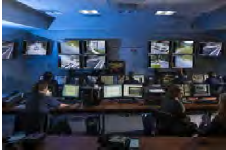
Figure 4.2: This photograph shows conventional surveillance interface where multiple monitors are placed in front of the operators. One of the greatest challenges for the users is to mentally fuse and interpret moving entities from multiple camera views.
