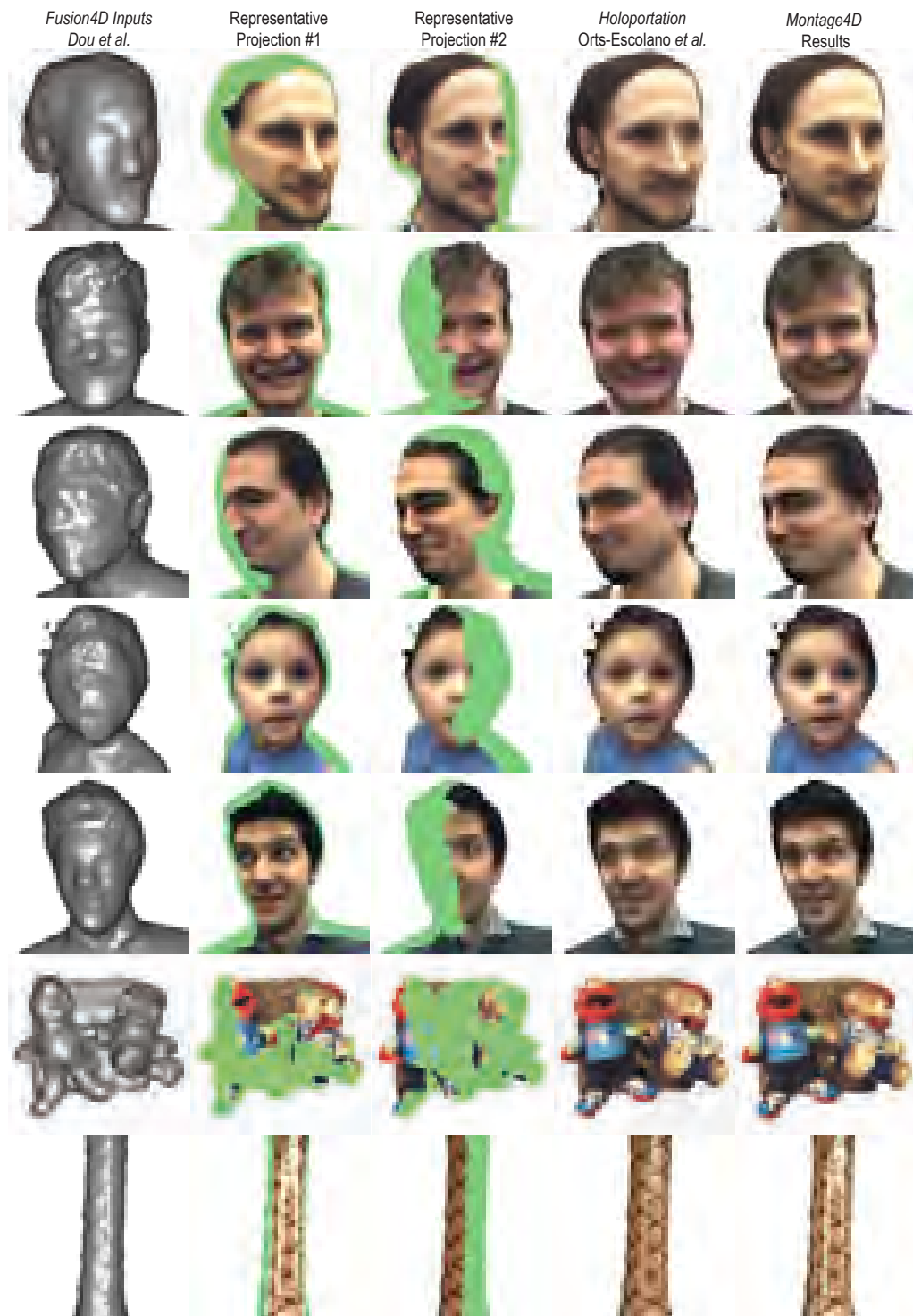
Figure 6.9: Comparison with the Holoportation approach. From left to right: the input mesh generated by Fusion4D, two representative back-projected images, and the rendering results from Holoportation and our Montage4D system.
