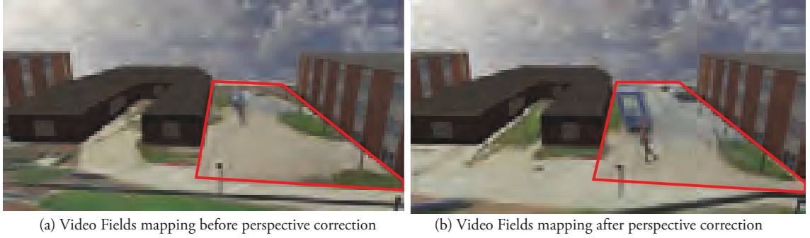
Figure 4.6: This figure shows the results before and after the perspective correction. The texture in (a) has the same perspective as the original video, but is not projected correctly in the 3D scene.
