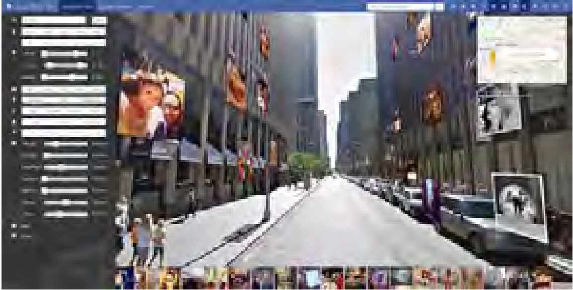
Figure 2.5: The Social Street View interface powered by WebGL and WebVR. The top navigation bar allows the user to switch among desktop and VR mode, input addresses, and enabling different postprocessing modes. The left control panel allows the user to search for certain keywords, filter based on the month of the year, the day of the week, and the distance to the current location. The top left legend shows a mini-map indicating where the user is located. The bottom panel is a baseline 2D approach for displaying nearby social media.
