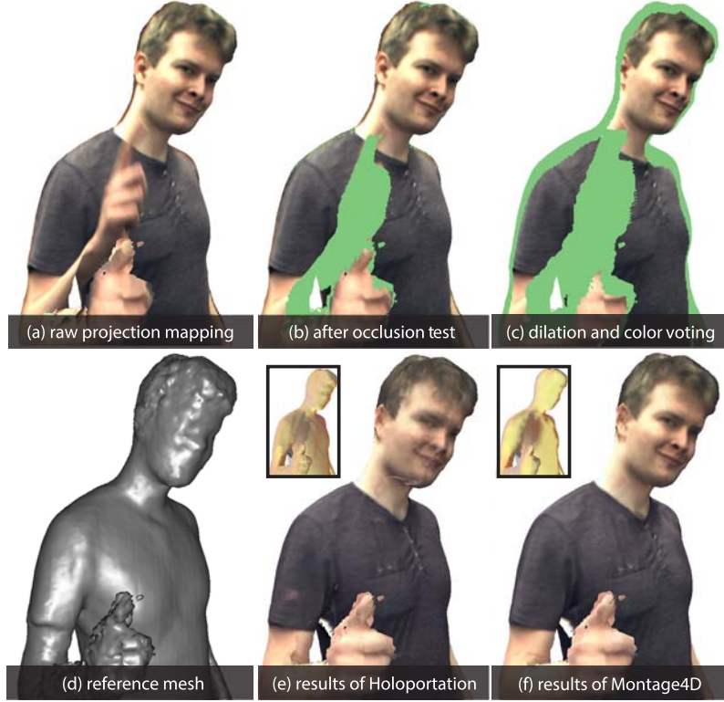
Figure 3. This figure shows how texture weight fields improve the rendering quality compared to the baseline approach. Holoportation removes several ghosting artifacts by taking advantage of dilated depth maps and majority voting algorithm (top row), however, the rendering still suffers from fuzziness and visible seams (bottom row). (a) shows the raw projection mapping result from an input video texture, (b) shows the culling result after the occlusion test, (c) shows the culling result after using dilated depth maps and majority voting algorithm, (d) shows the input mesh, (e) and (f) respectively shows the rendering results from the baseline approach and our algorithm, together with the corresponding texture weight fields for comparison.
