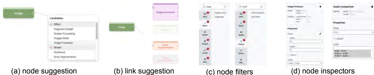
Figure 7: Examples of Rapsai's node-graph editor and inspectors: (a) when the user drag-and-drops an edge from a node to blank area in the editor, Rapsai automatically suggests a list of compatible nodes; (b) invalid nodes are greyed out to prevent users from programming errors; (c) users can filter nodes with keywords in the node library; (d) users can change node properties on the rightmost node inspector panel.
