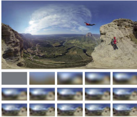
FIGURE 3. Reconstructed images using the first 15 frequency bands of SH coefficients extracted from the video frame.
