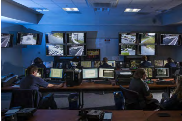
Figure 2: This photograph shows conventional surveillance interface where multiple monitors are placed in front of the operators. One of the greatest challenges for the users is to mentally fuse and interpret moving entities from multiple camera views.
