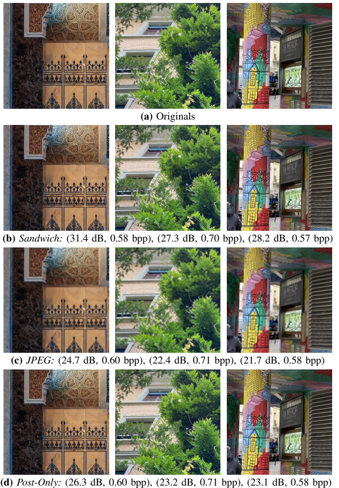
Fig. 2. Super-resolution sandwich: Original 256 \times 256 source images and reconstructions by sandwich, JPEG with linear upsampling, and JPEG enhanced with neural post-processing respectively. With the sandwich visually relevant ornaments/textures are preserved, images are sharper in a way that matches the originals, and text in the scene is easier to read. Beyond significantly improved visual quality the sandwich obtains substantial dB improvements (+5.1 dB, +4.1 dB, +5.1 dB over neural post-processing) at the same rate.
